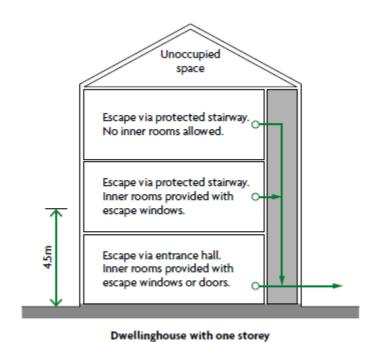
General means of escape in case of fire routes for a building with a new second floor
