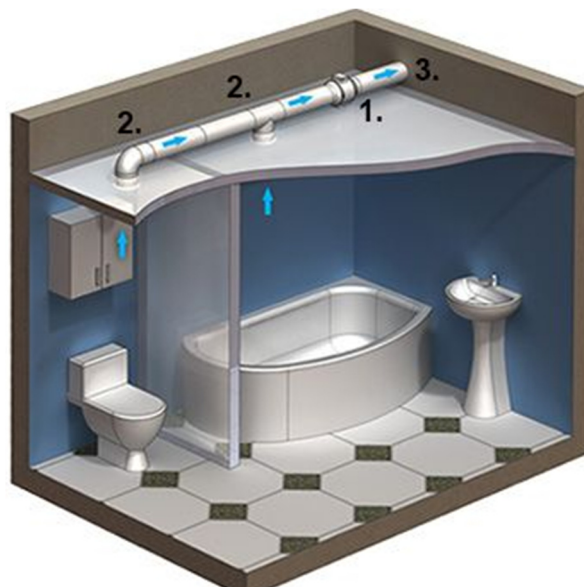
Image 5. Showing extract fan positions (2) extracting stale or moist air to the outside air.
